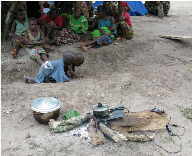
Figure 4: Charging a phone with the Hatsuden Nabe
