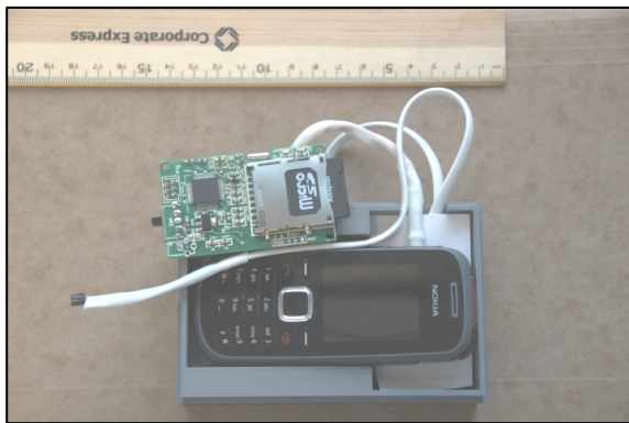
Figure 2: FoneAstra with a temperature sensor (at the end of the white cable used to place it appropriately within the cold-box) and connected to a Nokia 1661 mobile phone. The SD card is visible on the right side of the FoneAstra board. The ensemble is packaged in the gray box visible around the phone (the final dimensions are 12cm X 8cm X 5cm).
