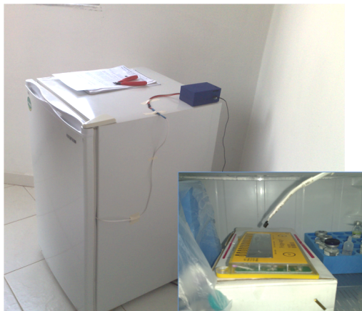
Figure 6: FoneAstra deployed at a health center. Note the box on the top back-right corner of the household fridge and the wire going down to the door and through the insulating lining. The inset shows the sensor hanging inside the fridge, just above a FridgeTag for comparing temperature readings from both devices.
