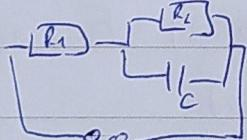
$$\frac{1}{Z_{N1}} = \frac{1}{R_2} + \frac{1}{i\omega C} = \frac{1 + i\omega RC}{R} \Rightarrow Z_{N1} = R \frac{1 - i\omega C}{1 + \omega^2 C^2}$$
