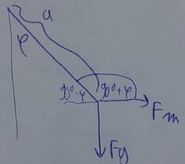
$$\alpha' mg \sin(180^\circ - \varphi) = I \cdot l \cdot B \cdot \alpha' \sin(90^\circ + \varphi) \quad 5$$
