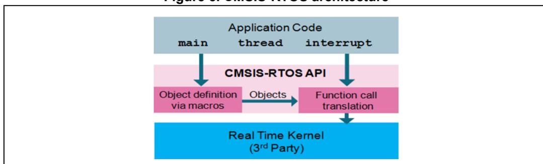
A typical CMSIS-RTOS API implementation interfaces to an existing Real-Time Kernel. The CMSIS-RTOS API provides the following attributes and functionality:
