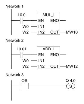
The MUL\_I box is activated by signal state "1" at I0.0. The ADD\_I box is activated by logic "1" at I0.1. If the result of one of the math functions was outside the permissible range for an integer, the OS bit in the status word is set to "1". Q4.0 is set if the scan of OS is logic "1".
