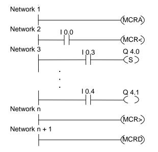
MCR functionality is activated by the MCRA rung. The rungs between the MCR< and the MCR> (outputs Q4.0, Q4.1) are executed as follows:
