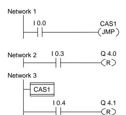
If 10.0 = "0", the jump to label CAS1 is executed. Because of the jump, the instruction to reset output Q4.0 is not executed even if there is a logic "1" at 10.3.
