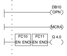
The Ladder rungs shown above are program sections from a function block written by a user. In this FB, DB10 is opened and MCR functionality is activated. If the unconditional call of FC10 is executed, the following occurs:
