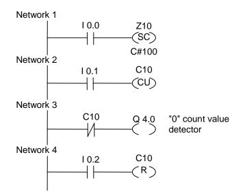
If the signal state of input I0.0 changes from "0" to "1" (positive edge in RLO), the preset value of 100 is loaded to counter C10.
