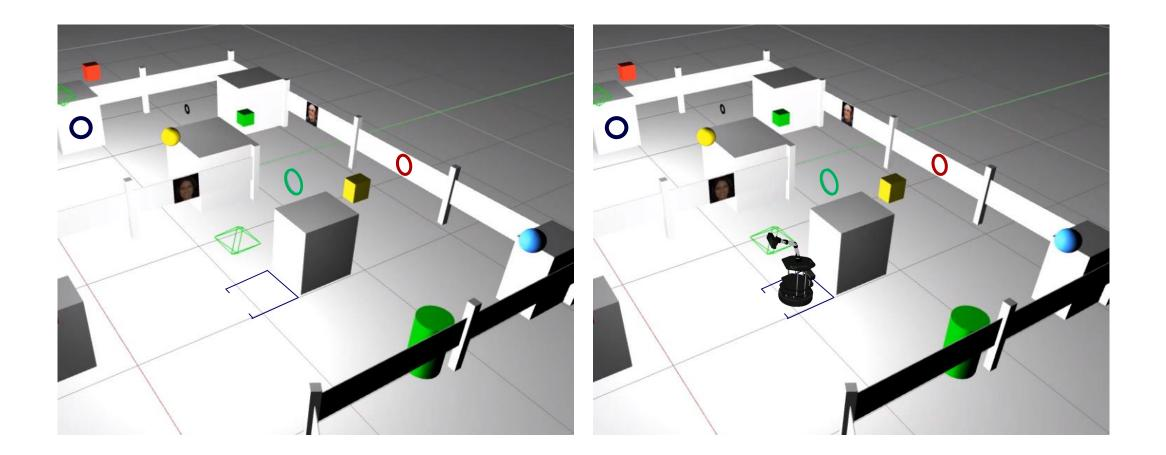
The robot should be positioned completely within the boundaries of the parking space
