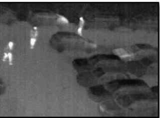
Long-wavelength infrared "light" (FLIR)
